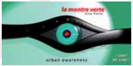
The "Montre Verte", which is designed to be worn by people in cities, captures, stores and measures data that are published on a dedicated network. The device is equipped with environmental sensors (measuring ozone and noise), as well as a GPS chip and Bluetooth system. The "Montre Verte" is connected to a cell phone that collects and transfers data to a web platform (Citypulse). This, in turn, converts the data flows into maps accessible to everyone that can be useful on a day-to-day basis.
